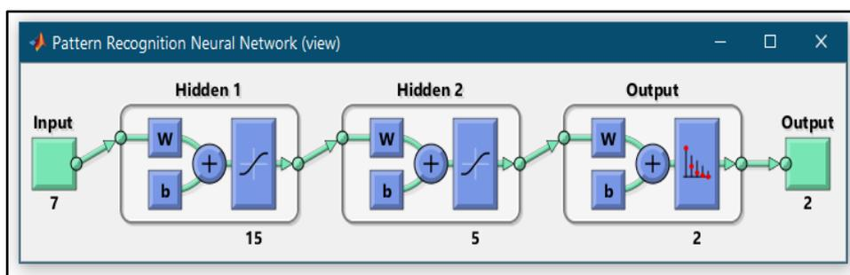
Figure 6. Structure of proposed BPN.
