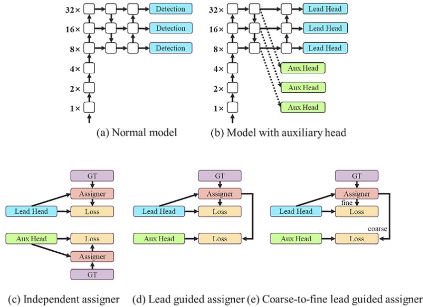
Figure 7. Coarse-to-fine auxiliary head supervision in the YOLOv7 [33]
