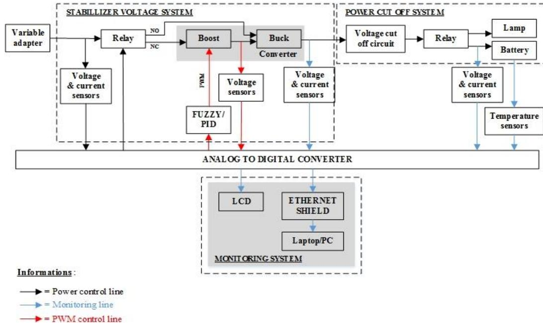
**Figure 2.** Block Diagram of Voltage Stabilizer Prototype for Battery Charging
