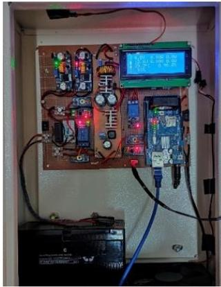
**Figure 9.** Physical of Voltage Stabilizer Prototype for Battery Charging
