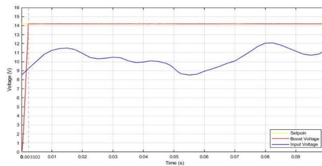
**Figure 10.** Simulation Results of Boost Converter Using Fuzzy Logic
