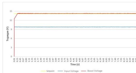
**Figure 11.** Results of Hardware Implementation of Boost Converter Using Fuzzy Logic Control
