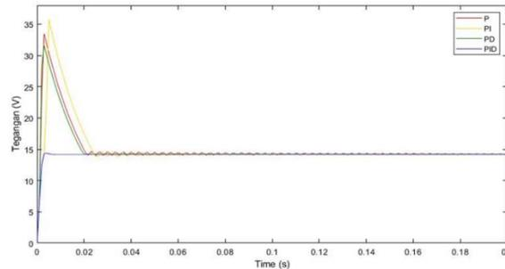
Figure 12. Simulation Results of PID Using Ziegler-Nichols
