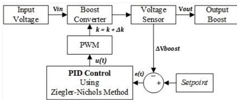
Figure 8. Block Diagram of PID Control Implementation on Boost Converter
