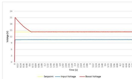
Figure 13. Implementation Results of the Output Boost Converter Using PID Control
