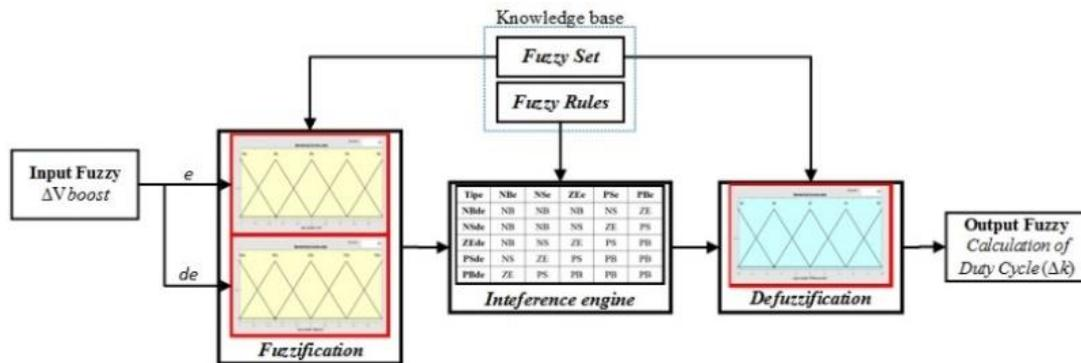
Figure 5. Structure of the Fuzzy Logic Control
