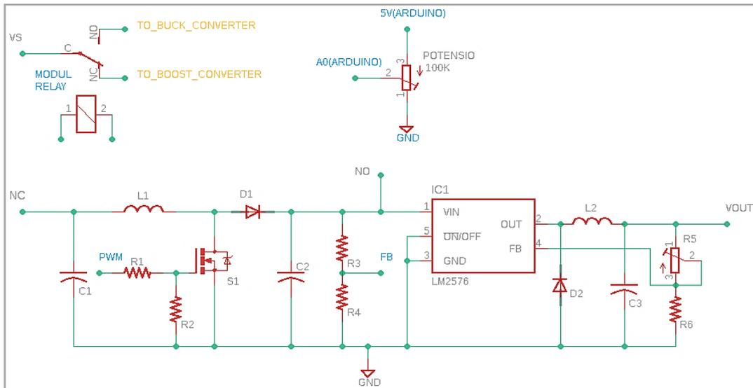
**Figure 3.** Boost-Buck Converter Circuit Schematic
