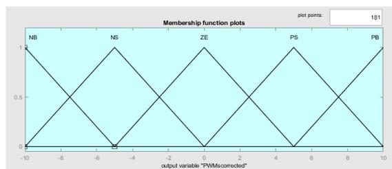
Figure 7. Membership function of PWM's corrected ( $\Delta k$ )
