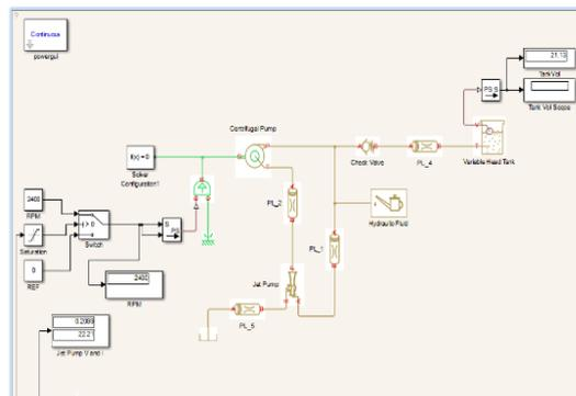
Figure 6. Block Diagram of Water Jet Pump
