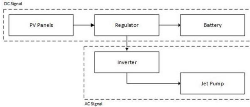
Figure 1. Simplified Block Diagram of PV Panel DC-AC Converter System
