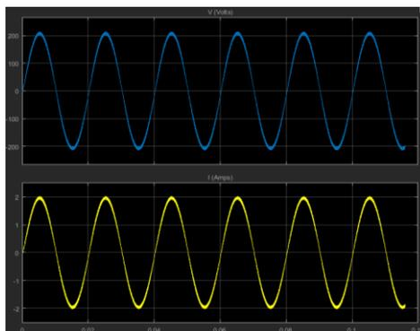
Figure 5. Output Signal From DC-AC Converter
