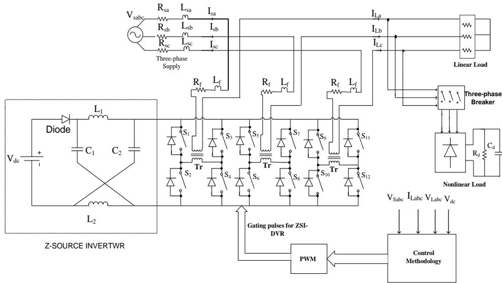
Figure 3. Schematic Diagram of Proposed ZSI-DVR
