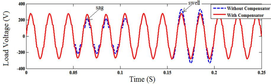
Figure 13. Load Voltage with and without CSI-DVR
