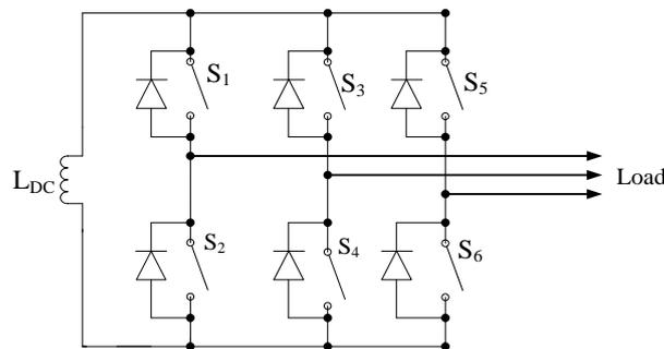
Figure 5. Basic Configuration of Current Source Inverter
