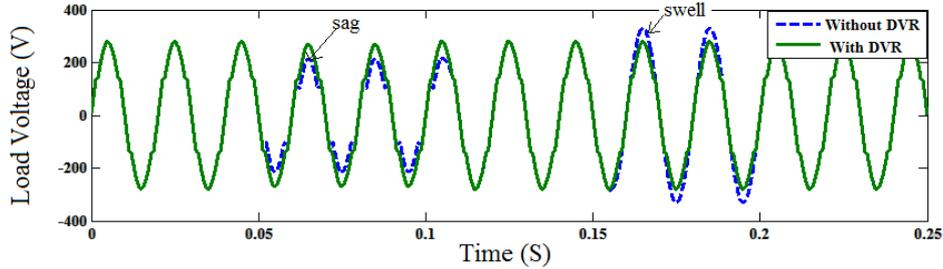
Figure 15. Load Voltage with and without ZSI-DVR
