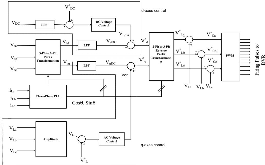
Figure 9. Block Diagram of D-Q Control Technique
