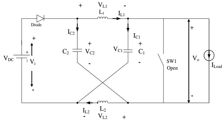
Figure 8. Shoot-Through Wtate of Z-Source Inverter
