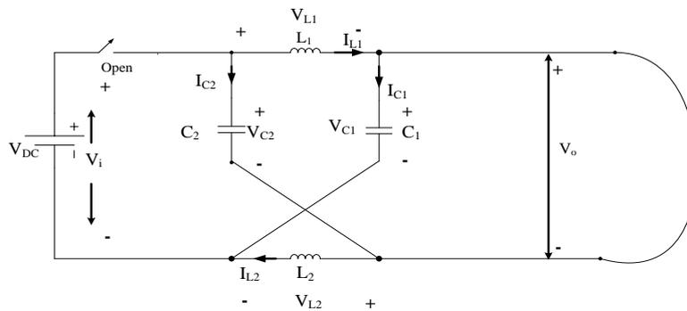
Figure 7. Active and Zero State of Z-Source Inverter
