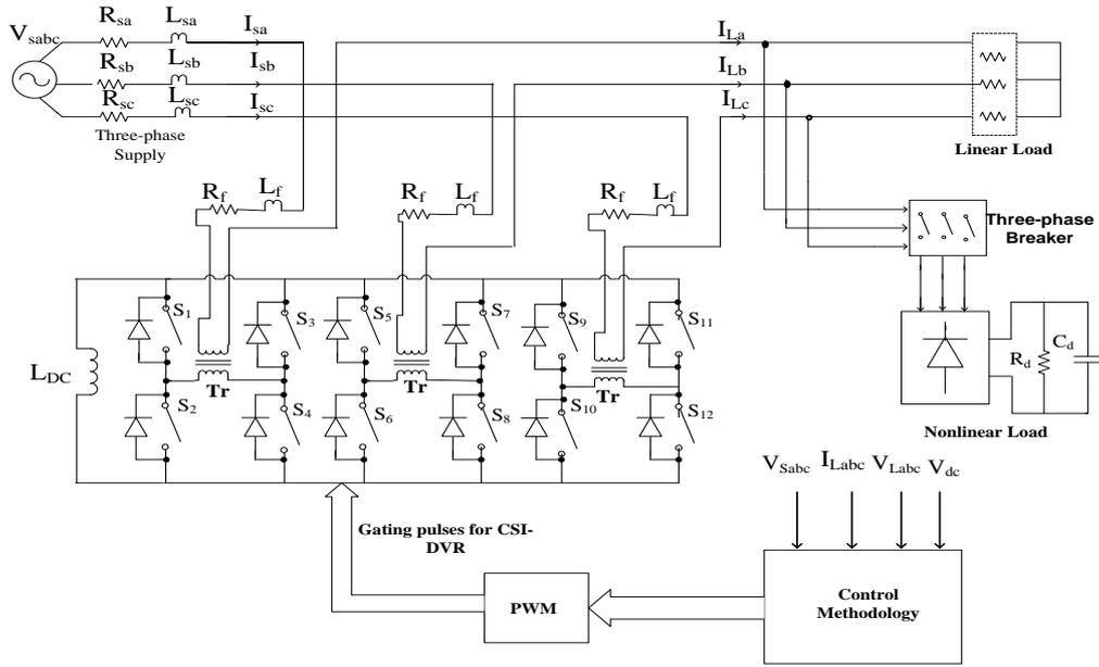
Figure 2. Schematic Diagram of Traditional CSI-DVR
