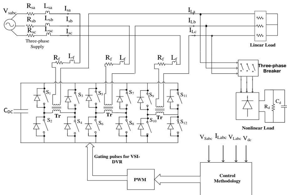
Figure 1. Schematic Diagram of Traditional VSI-DVR
