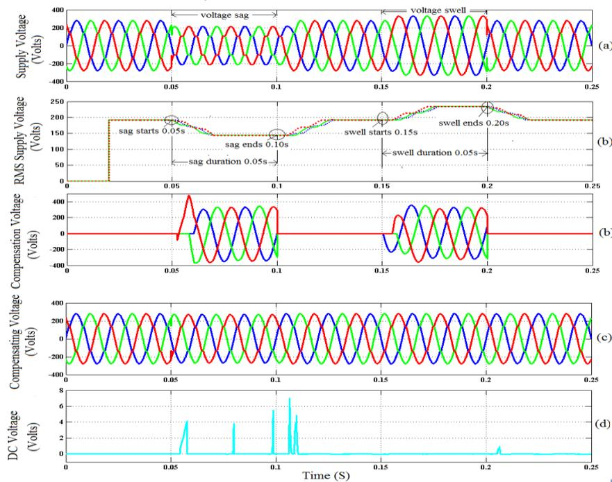
Figure 12. Simulation Results of CSI-DVR (a) Supply Voltage (b) RMS Supply Voltage (c) Injected Voltage of CSI-DVR (d) Load Voltage and (e) DC-link Voltage
