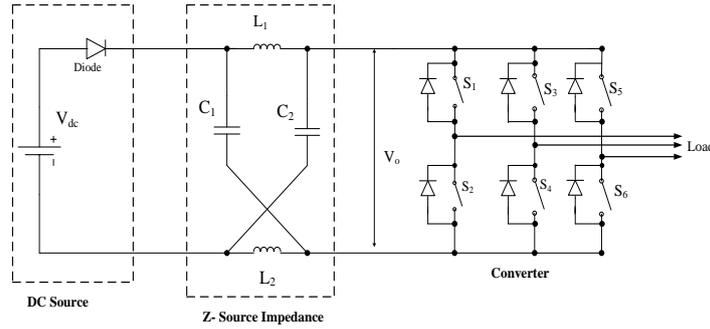
Figure 6. Basic Configuration of Z-Source Inverter
