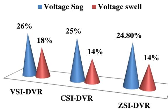
Figure 17. Measured Chart for Voltage Sag/Swell by VSI-DVR, CSI-DVR and ZSI-DVR
