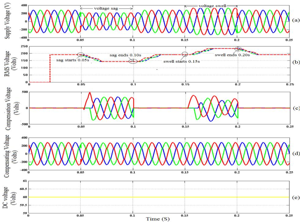
Figure 14. Simulation Results of ZSI-DVR (a) Supply Voltage (b) RMS Supply Voltage (c) Injected Voltage of ZSI-DVR (d) Load Voltage and (e) DC-link Voltage
