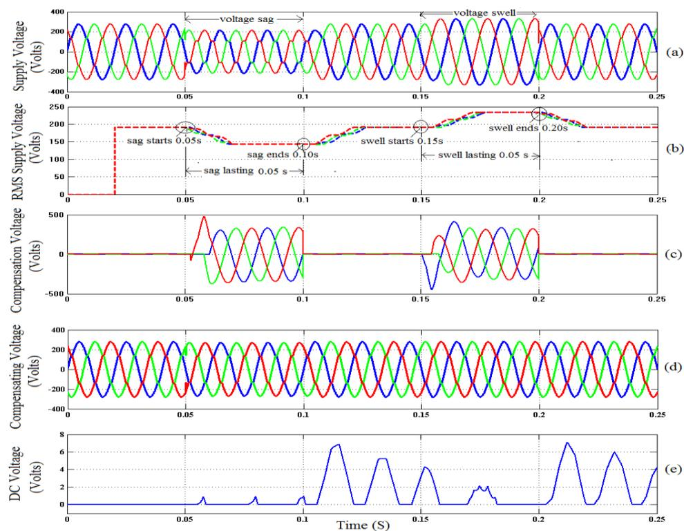
Figure 10. Simulation Results of VSI-DVR (a) Supply Voltage (b) RMS Supply Voltage (c) Injected Voltage of VSI-DVR (d) Load Voltage and (e) DC-link Voltage
