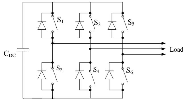
Figure 4. Basic Configuration of Voltage Source Inverter
