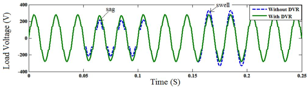
Figure 11. Load Voltage with and without VSI-DVR
