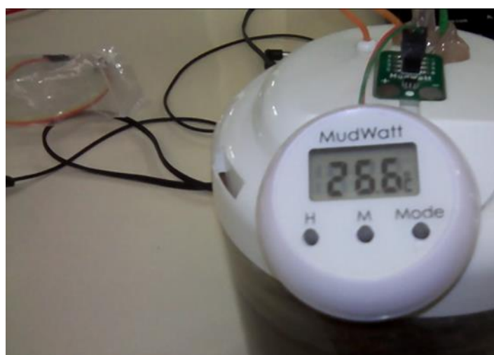
Figure 3. Temperature sensor being powered by the Microbial Fuel Cell
