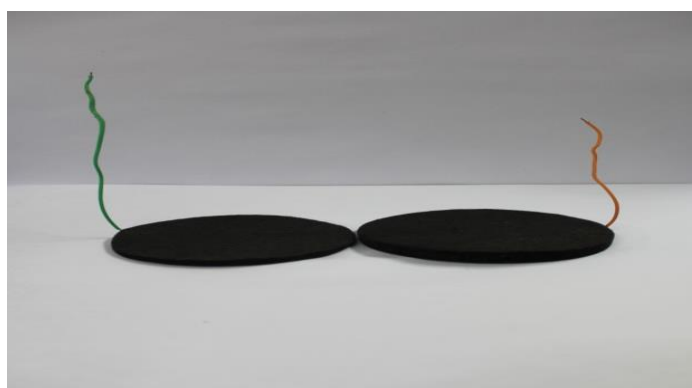
Figure 1. The graphene based anode on the right and cathode on the left
