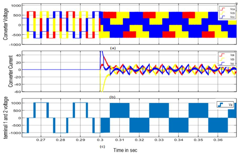
Figure 5. Simulation waveform of the STATCOM power converter output terminals (a) converter output voltage, (b) STATCOM converter output compensating current (c) waveforms of the AC voltages generated by inverter 1 (legs 1 and 3).
