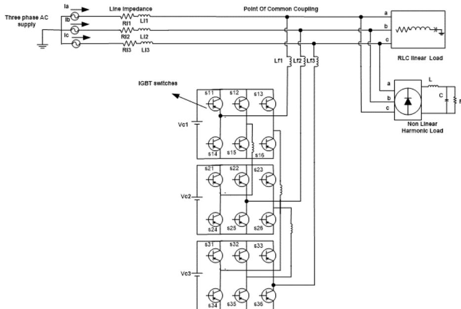
Figure 1. Block diagram of proposed STATCOM module
