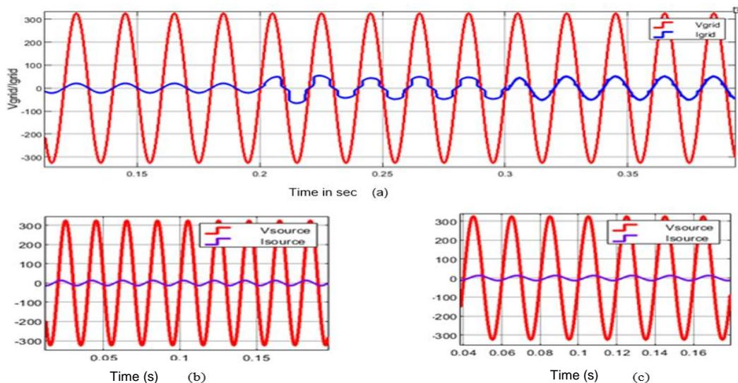
Figure 7. (a) Waveforms of the grid voltage and grid current with and without STATCOM in the system. (b)Capacitive mode of operation, and (c) Inductive mode of operation
