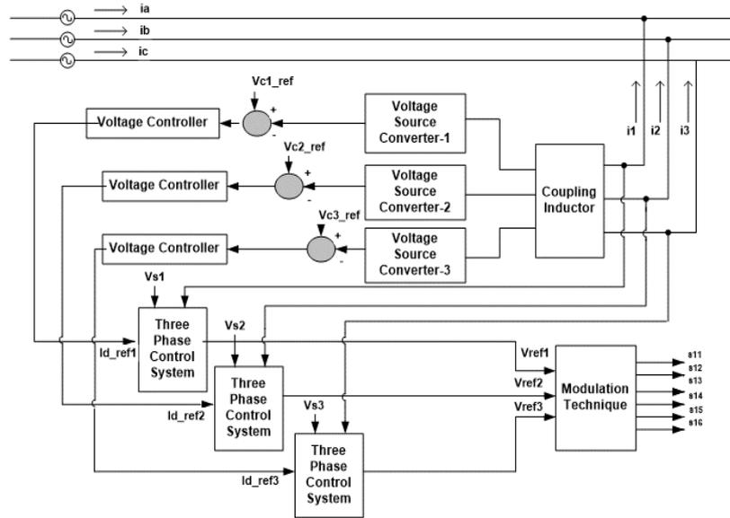
Figure 2. Control system for proposed STATCOM module
