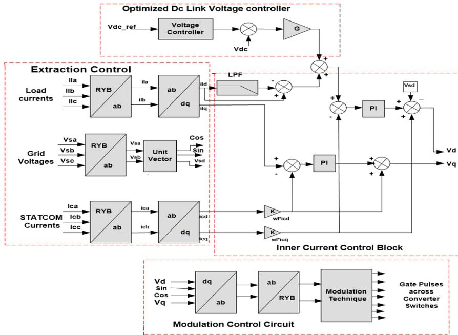
Figure 3. Control Circuit block diagram
