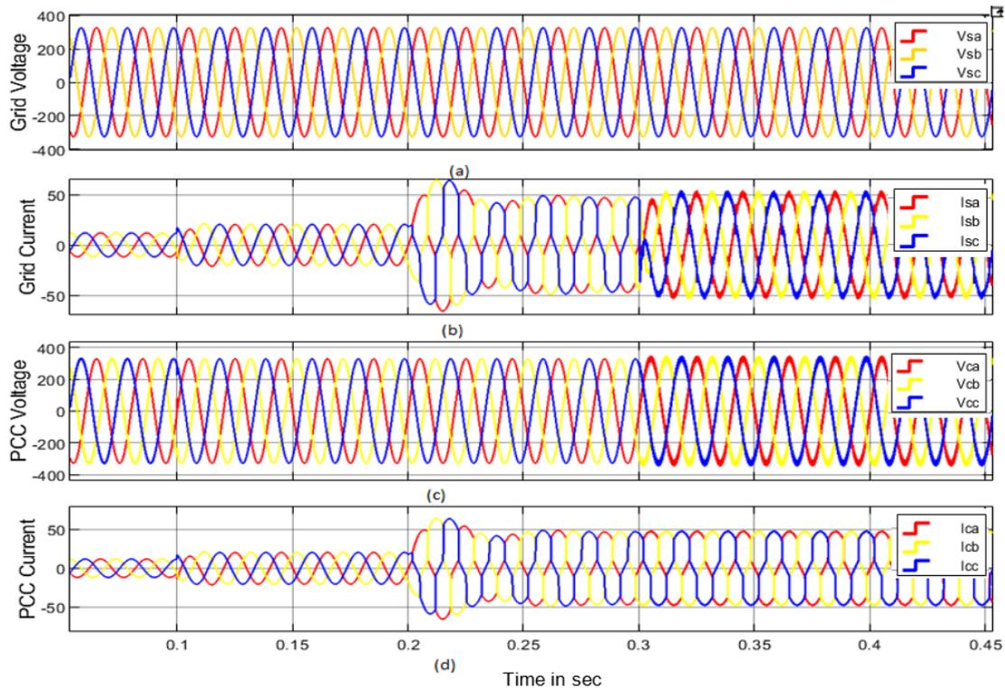
Figure 4. Simulation waveform of three phase (a) grid voltage, (b) grid current, (c) PCC voltage and (d) PCC current
