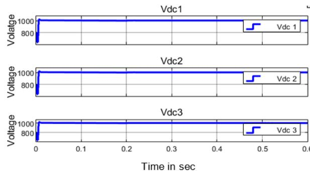
Figure 6. DC- link Capacitor voltage waveform across all cascaded converters with STATCOM.
