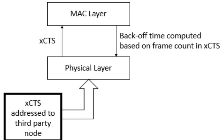
Figure 5. Calculation of back-off time based on frame count in xCTS
