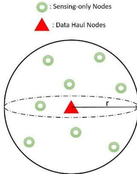
Figure 3. A single cluster consisting of sensing nodes and one data haul node
