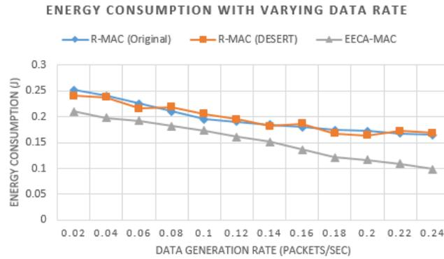
Figure 15. Energy consumption to transmit one packet
