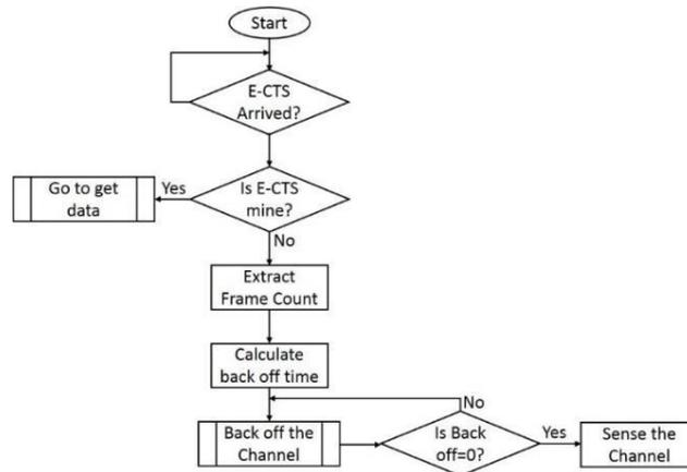
Figure 9. Sensing xCTS
