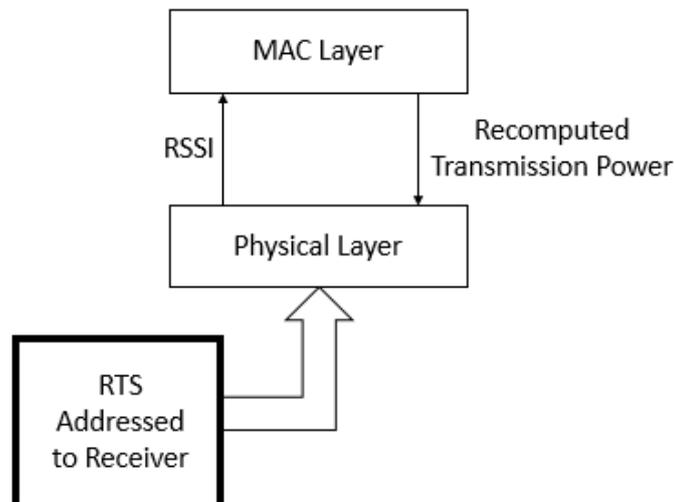
Figure 4. Adjustment of transmitter power based on RSSI at receiver
