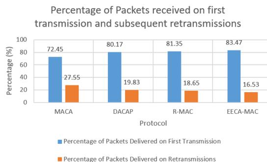
Figure 11. PDR for packets received on the first transmission and subsequent retransmissions
