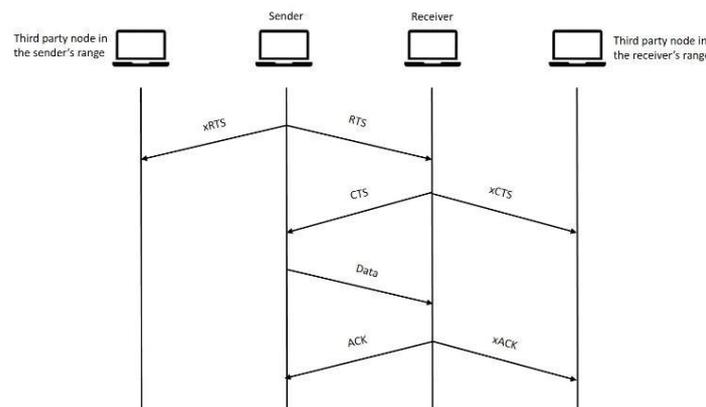
Figure 2. Control packet exchange of MACAW
