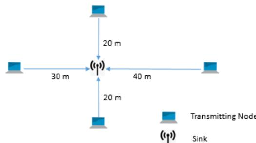
Figure 14. Network Topology-2 for per-packet energy consumption
