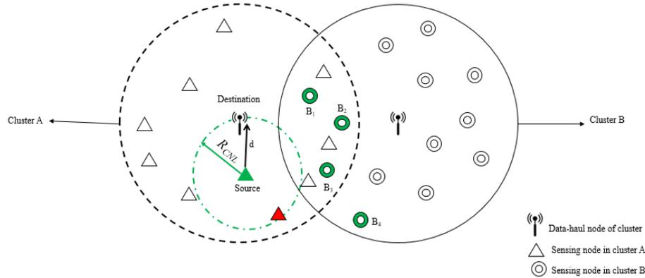
Figure 23. Interference range of source node using adaptive power control
