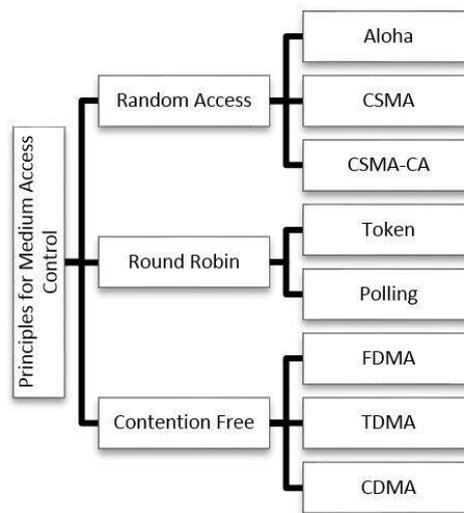
Figure 1. Principles of medium access control
