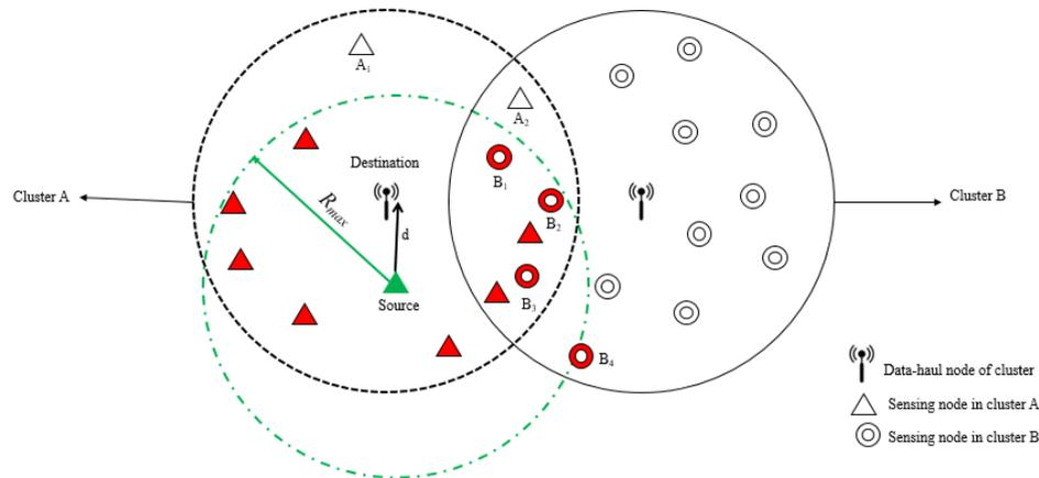
Figure 22. Interference range of source node without adaptive power control
