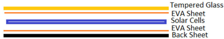
Figure 3. PV Panels layout
