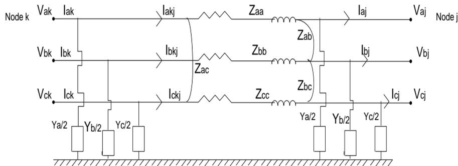
Figure 1. Representation of line model between bus  $k$  and  $j$
