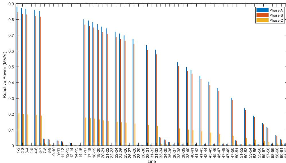
Figure 10. Reactive power losses of the Ajinde 62-bus network
