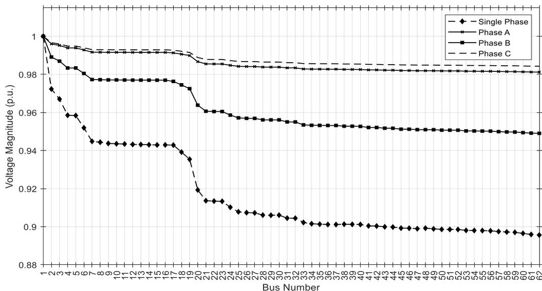
Figure 13. A comparison of the voltage profiles between single-phase and three-phase methods for Ajinde 62-bus network
