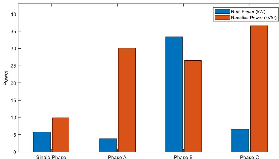
Figure 14. A comparison of the power losses between single-phase and three-phase methods for Ajinde 62-bus network
