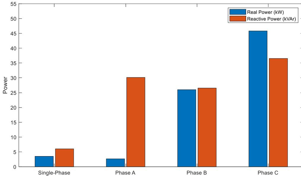
Figure 12. A comparison of the power losses between single-phase and three-phase methods for Olusanya 54-bus network
