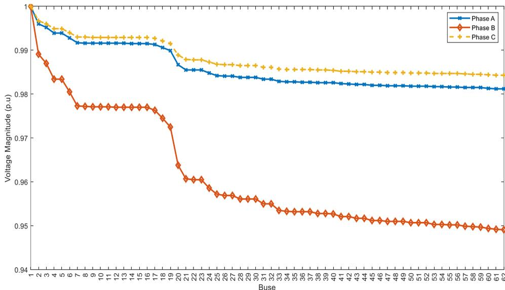
Figure 8. Voltage profile of the Ajinde 62-bus system
