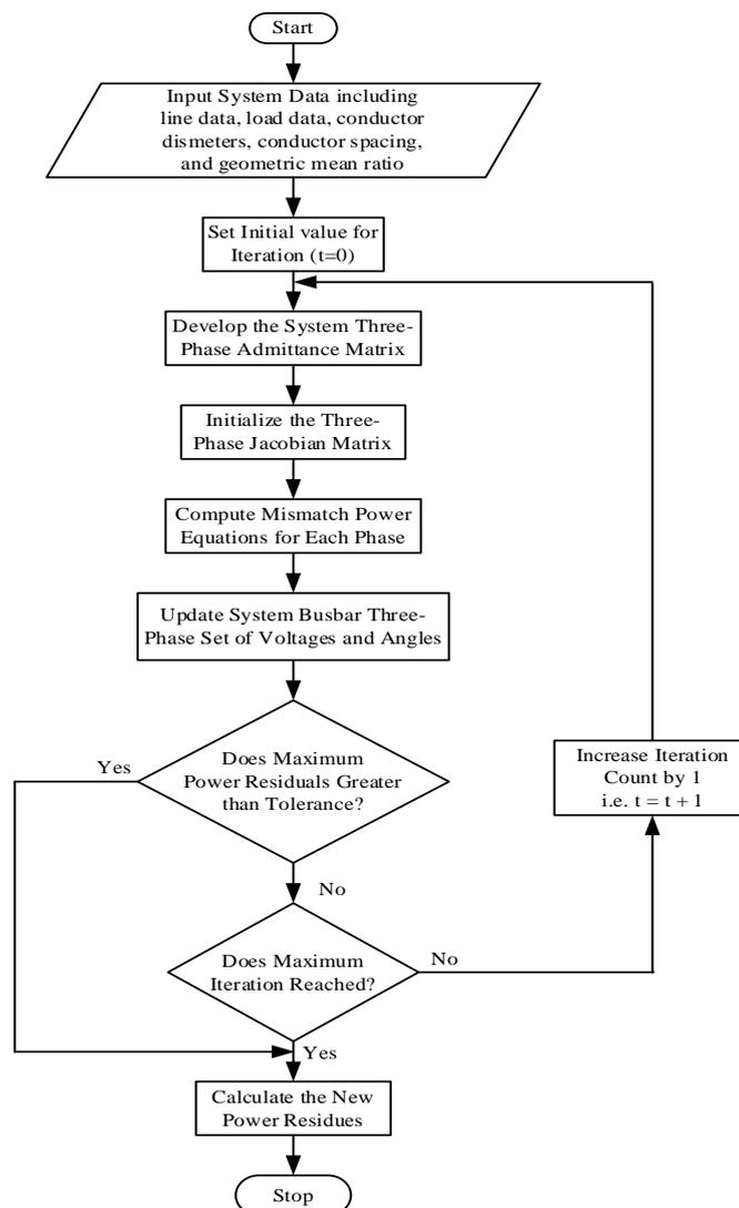
Figure 2. Flow chart for the three-phase Newton-Raphson power flow solution
