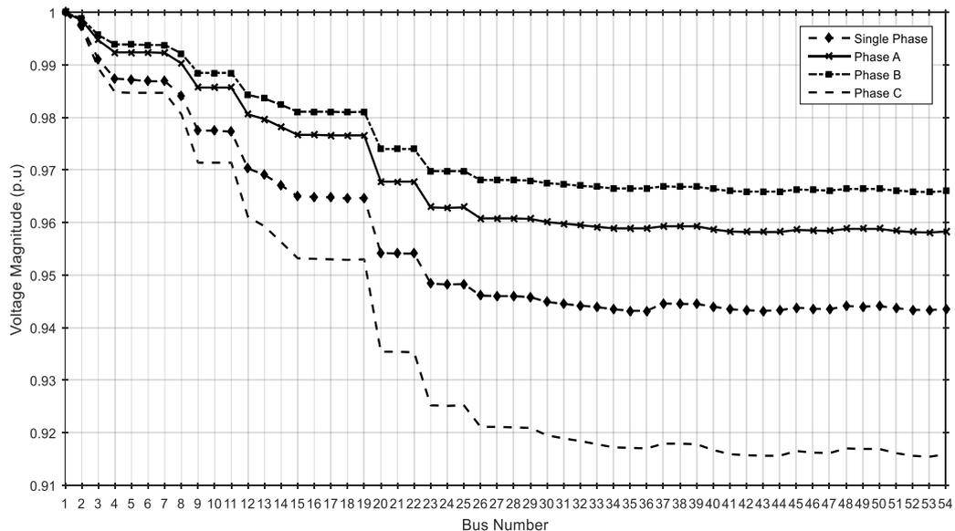
Figure 11. A comparison of the voltage profiles between single-phase and three-phase methods for Olusanya 54-bus network
