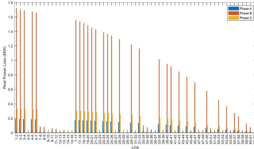
Figure 9. Real power losses of the Ajinde 62-bus network
