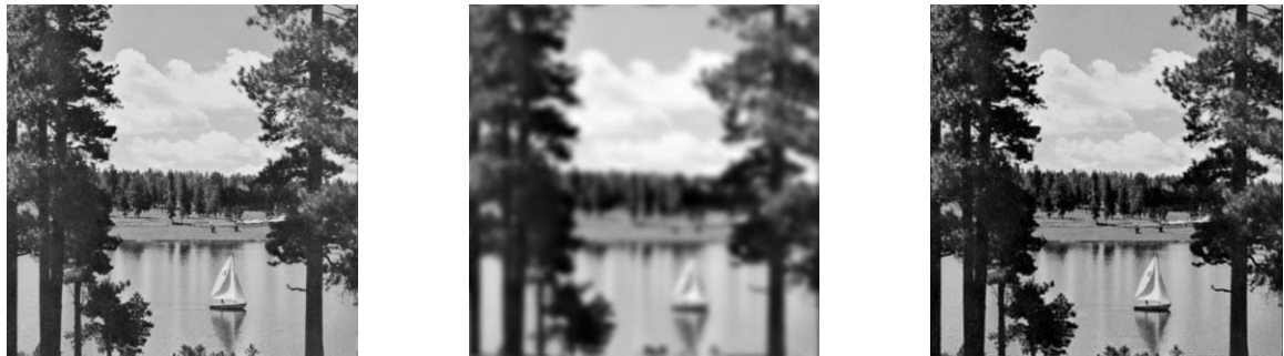
Figure 3. b. Lake image: before being blurred by a high amount of blur, after being blurred and the restored image using inverse filtering
