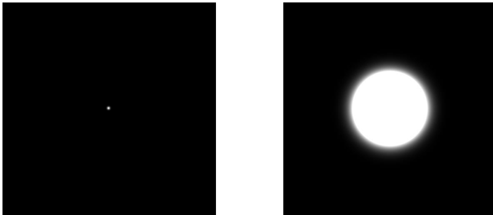
Figure 2. a. PSF and MTF for a medium quantity of blur in the inverse filtering stage of the proposed method
