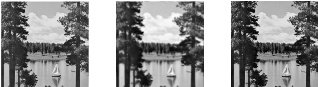
Figure 2. b. Lake image: before being blurred by a medium amount of blur, after being blurred and the deblurred image using inverse filtering
