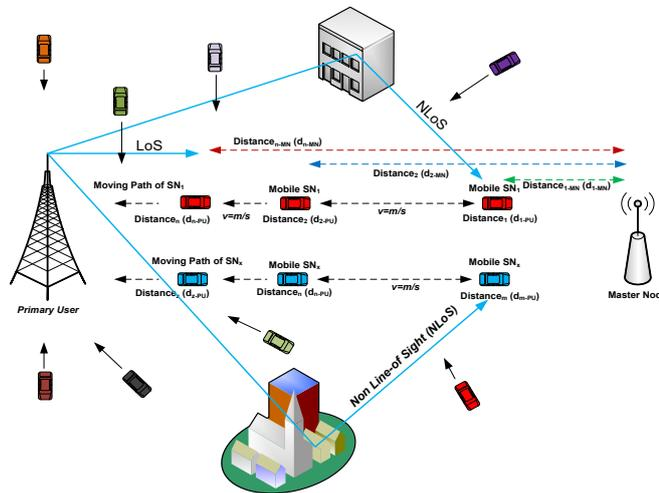
Figure 4. Scenario of Spectrum Sensing Information Exchange Method with SN mobility.
