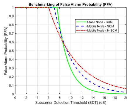
Figure 11. Benchmarking of False Alarm Probability (PFA) performance between static node SCM and mobile node SCM.
