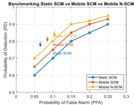
Figure 12. Receiver Operating Characteristic graph illustrating benchmarking results from Static SCM, Mobile SCM, and Mobile N-SCM, utilizing Probability of Detection (PD) and Probability of False Alarm (PFA) data.
