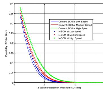
Figure 8. Probability of false alarm performance using different subcarrier mapping techniques at various SN velocities.
