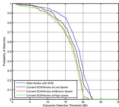
Figure 5. Probability of detection using *conventional Subcarrier Mapping* (SCM)
