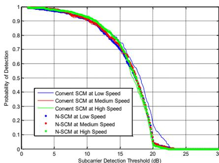
Figure 7. Probability of detection performance using different subcarrier mapping techniques at various SN velocities.
