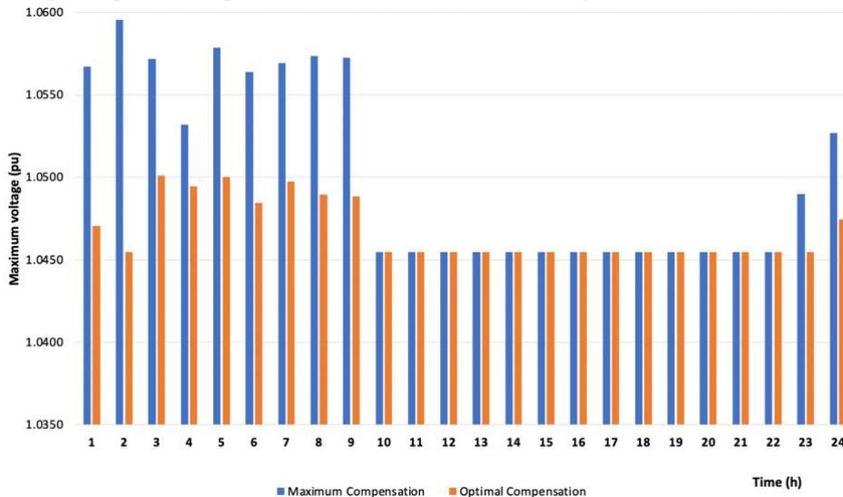
Figure 10. Maximum voltage curve in 2 cases: maximum compensation and optimal control compensation
