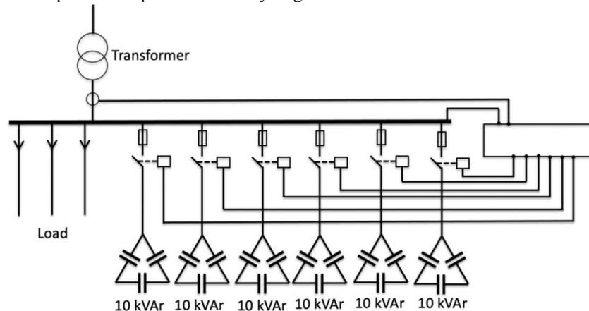
Figure 1. A switched capacitor banks of 60 kVar at a MV/LV substation
