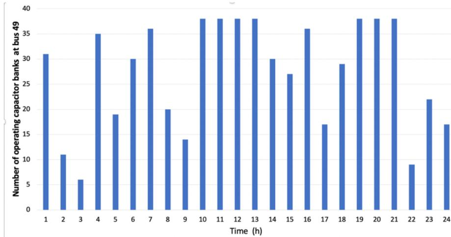
Figure 8. Number of capacitor banks switched on at bus 49
