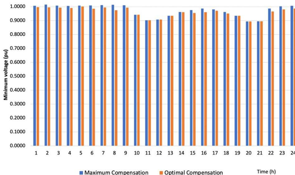
Figure 11. Minimum voltage curve in 2 cases: maximum compensation and optimal control compensation
