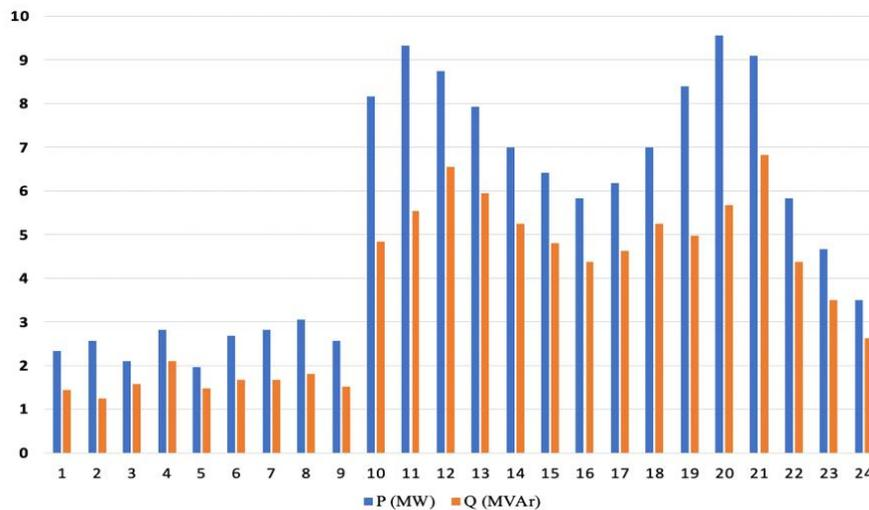
Figure 7. Total hourly active and reactive power load curve used for the modeling
