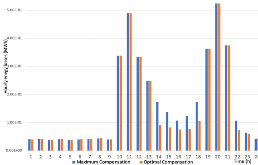
Figure 9. Power loss curve in 2 cases: maximum compensation and optimal control compensation
