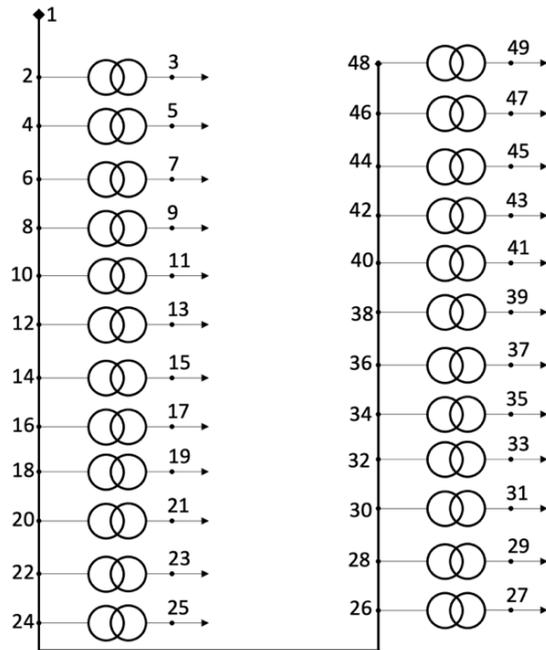
Figure 6. Single diagram of 22 kV distribution network modeling
