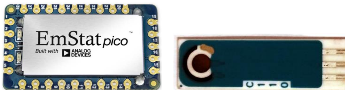
Figure 2. EmStat Pico [29] and the developed nanogold deposited biosensor
