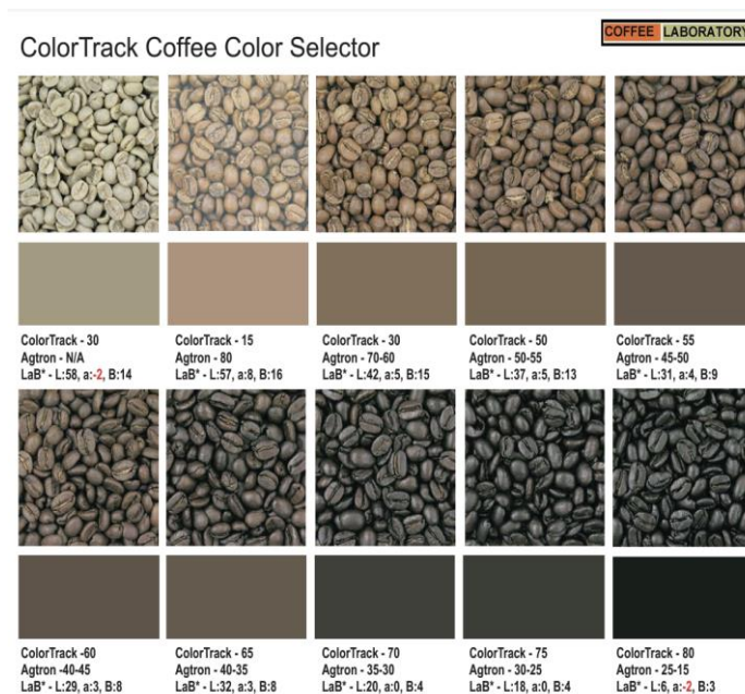
Figure 1. Agtron scale conversion to LAB color model [21]
