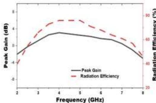
Figure 9. Peak Gain and Radiation Efficiency of the antenna.
