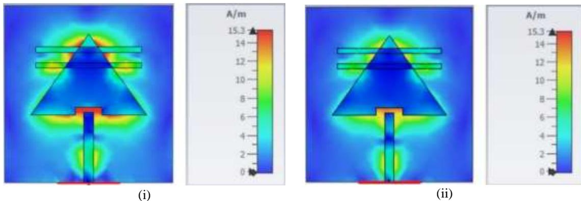
Figure 6. Simulated current density of the proposed antenna. i) 3.6 GHz and ii) 4.8 GHz.
