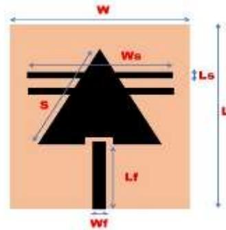
Figure 3. Design configuration of the designed antenna.
