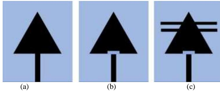
Figure 1. Design Evolution of the proposed antenna. a) Stage 1, b) Stage 2 and c) Stage 3.
