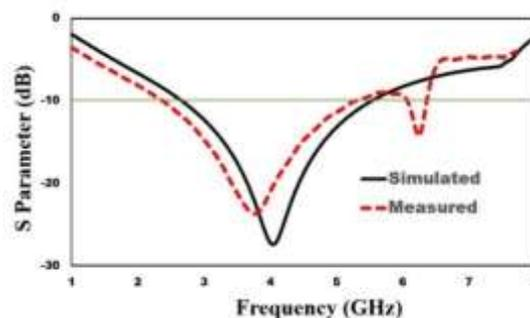
Figure 5. Combined reflection coefficients of the proposed antenna.
