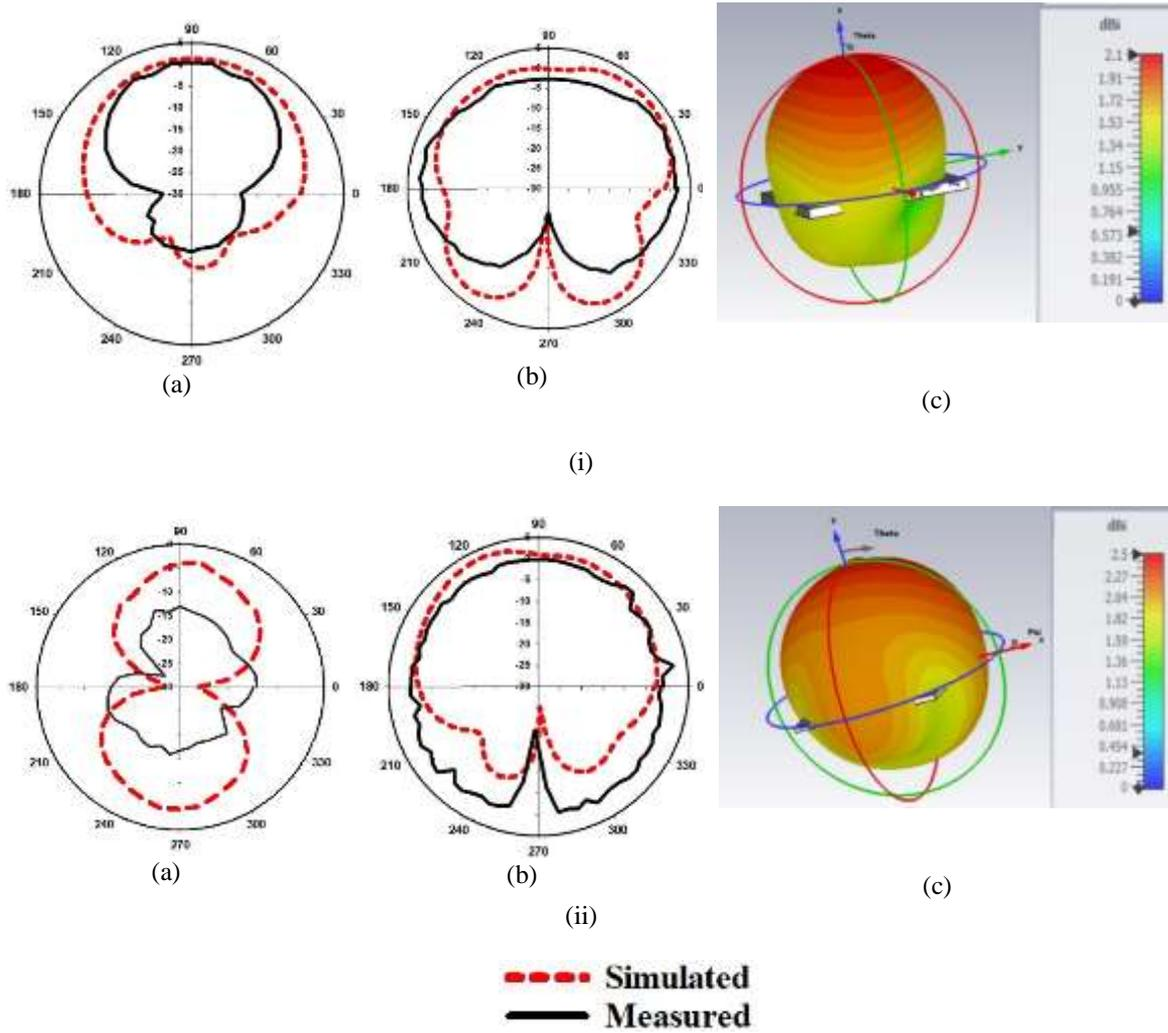
Figure 8. Combined radiation patterns of the designed antenna. a) E-plane, b) H-plane and c) 3-Dimensional, i) 3.6 GHz and ii) 4.8 GHz.
