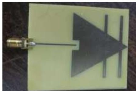
Figure 4. Fabricated prototype of the inset coupled-fed triangular patch antenna.
