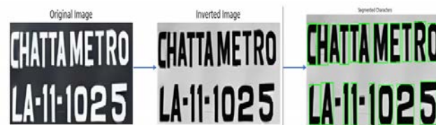
Figure 9. Inversion and Extraction for Black Colored Plates
