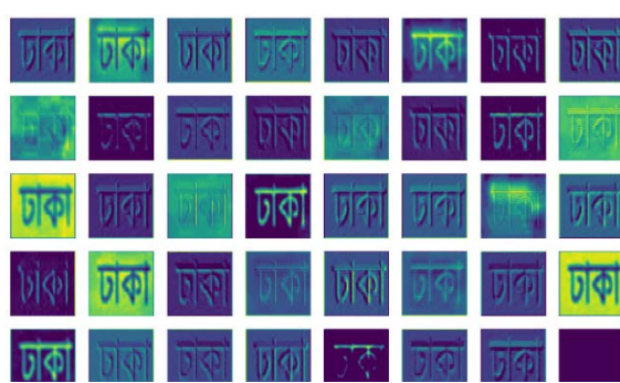
Figure 26. Feature Map from a layer of Bangla Number Plate Recognition Model
