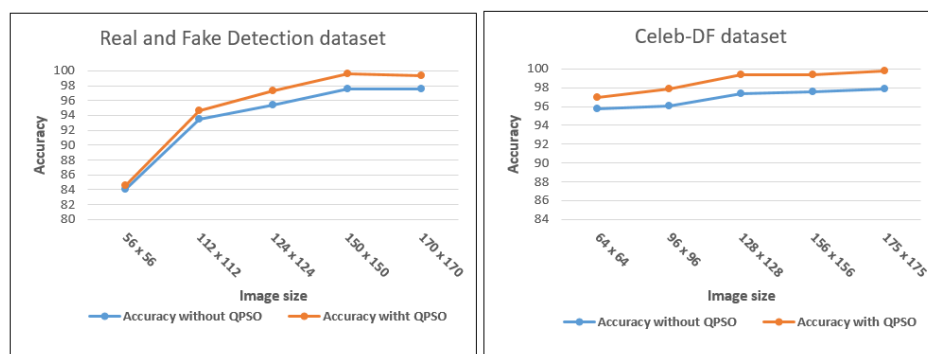
Figure 3. The performance at different image dimensions on "Real and Fake Detection" and "Celeb-DF" dataset
