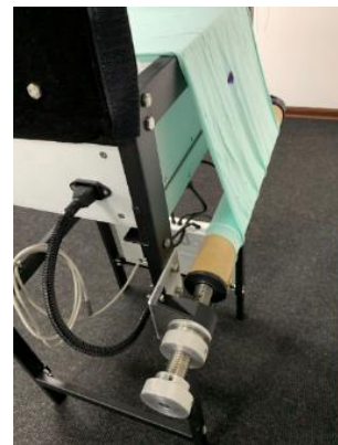
Figure 5. Fabric roll displacement system, rear view
