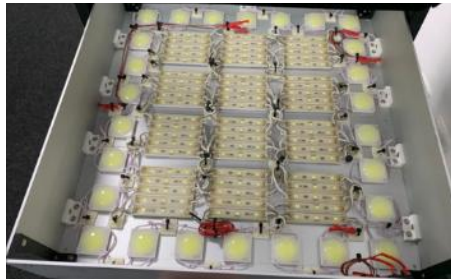
Figure 6. LEDs distribution for Back Light Illumination
