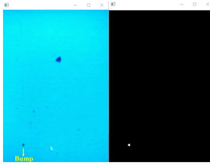
Figure 21. Left: Original Image. Right: Binarized image for bumps in light fabric
