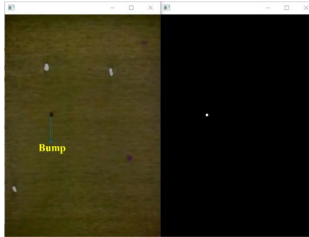
Figure 19. Left: Original Image. Right: Binarized image for bumps in dark fabric.
