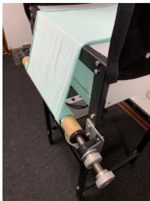
Figure 4. Fabric roll displacement system, front view
