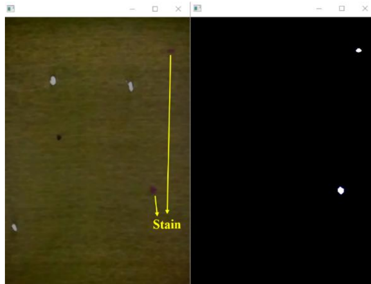
Figure 24. Left: Original Image. Right: Binarized image for stains in dark fabric
