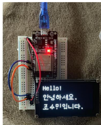
Figure 4. Hangul display with ESP32
