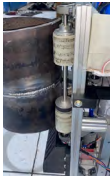
Figure 7. The procedure for capturing welding photos on sample pipes.
