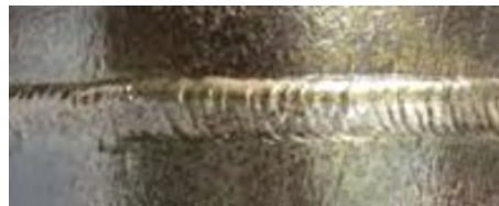
Figure 8. An example of a normal welding pattern on an iron pipe.
