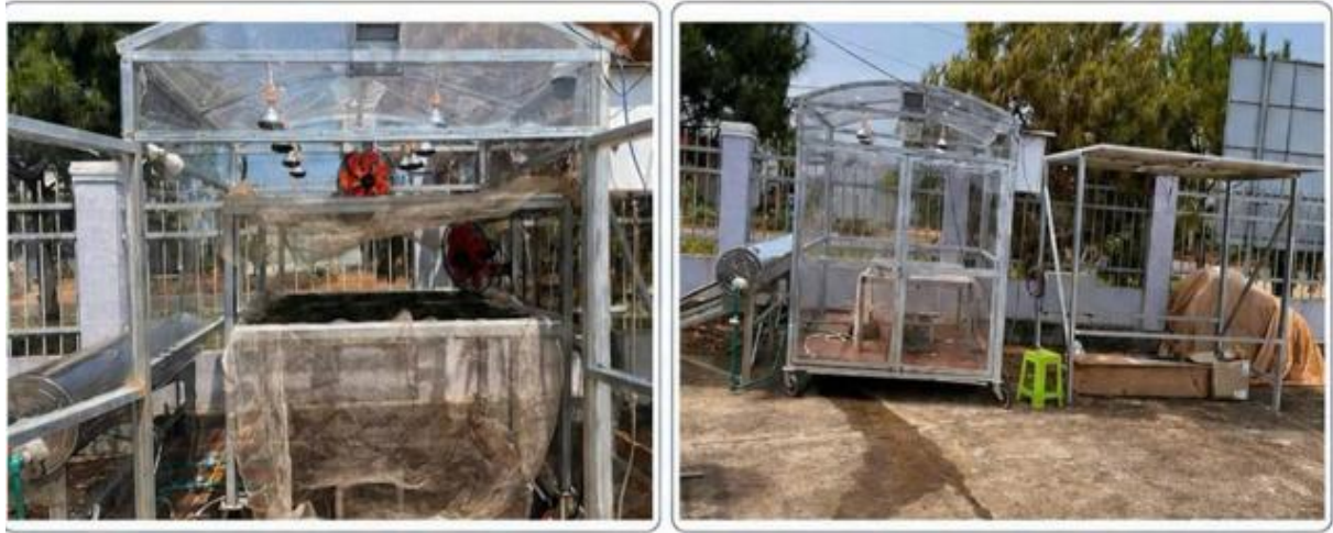
Figure 1. Experimental Drying System
