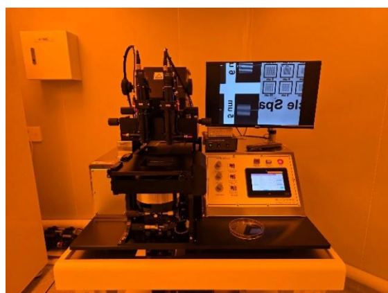
Figure 3. M150S Mask Aligner
