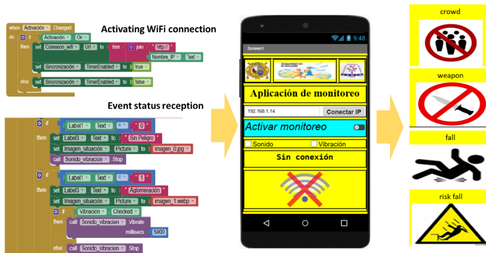
Figure 6. Activation block for receiving and configuring vibration and visual alarm
