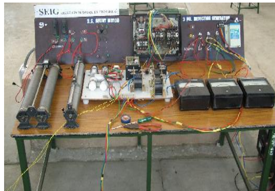
Figure 12. Photo graph of the D.C separately excited motor fed SEIG with R load
