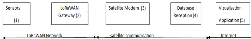
Figure 2. The architecture for the areas outside cellular network coverage
