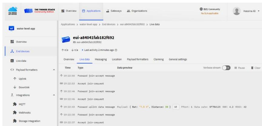
Figure 8. Connection of the LoRawAN Sensor on the Things Network through the 3G cellular network.
