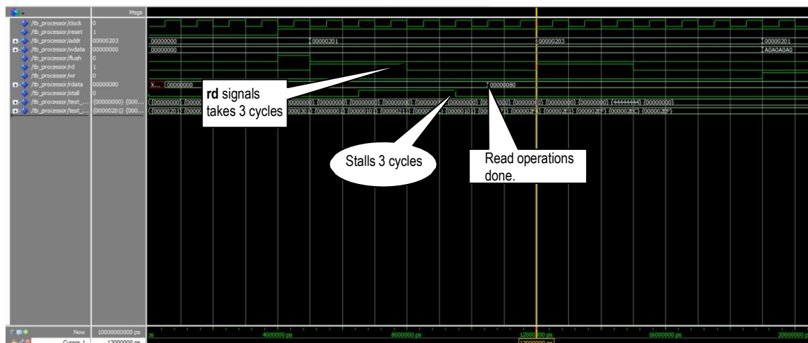
Figure 7. Simulation result of test_addr(0)=0000201 for the read miss.
