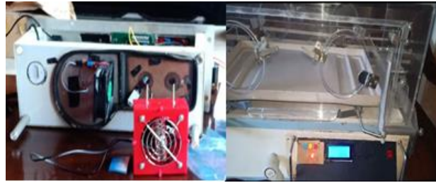
Figure 6. Chamber, heater, fan, fan sprayer, buzzer and valve
