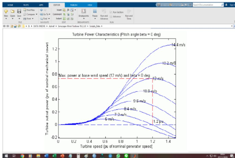
The illustration below shows the mechanical power  $P_m$  as a function of generator speed, for different wind speeds and for blade pitch angle  $\beta = 0$  degrees. This figure is obtained with the default parameters (base wind speed = 12 m/s, maximum power at base wind speed = 0.73 pu ( $k_p = 0.73$ ), and base rotational speed = 1.2 pu).
