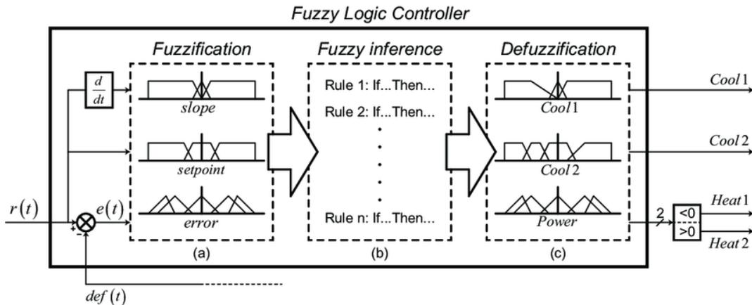
Figure 4.5. Output Value - Fuzzy Logic Controller 2
