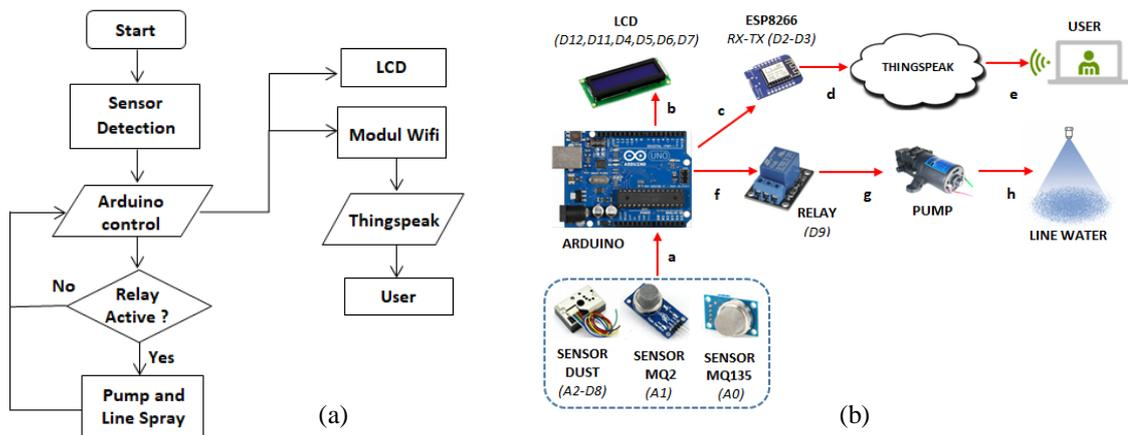
Figure 3. Flow Chart (a) and Block Diagram of Hardware Designing (b)
