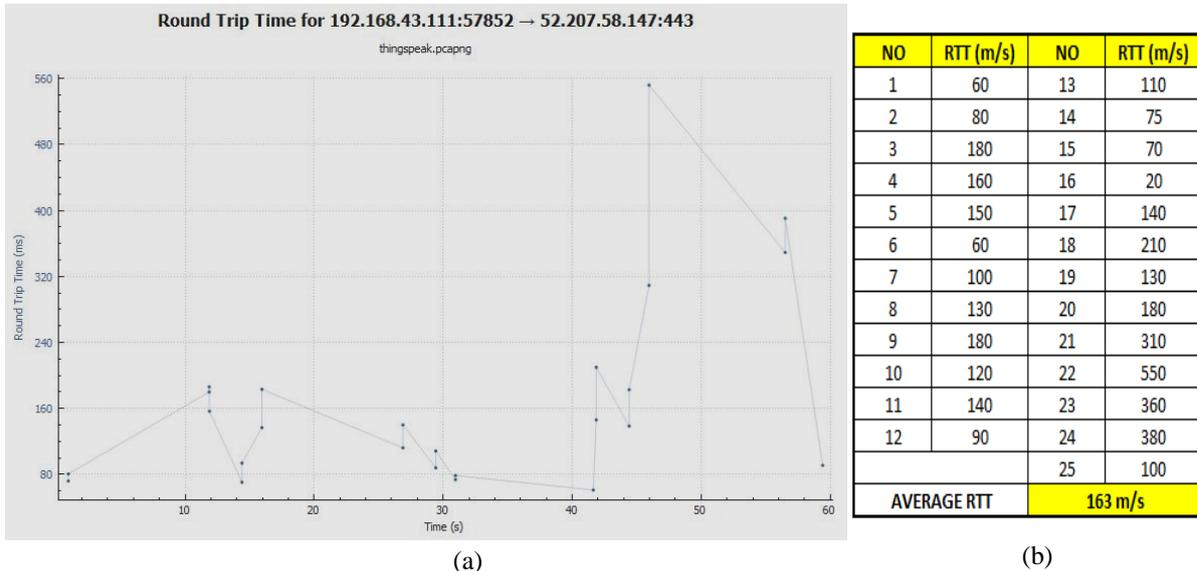
Figure 8. Graph (a) and RTT Measurement Table (b)
