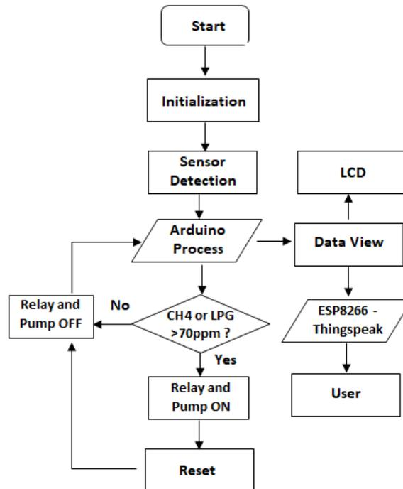
Figure 4. Flow Chart of Software Designing
