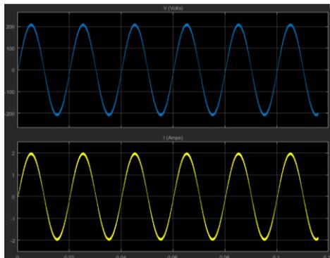
Figure 5. Output Signal From DC-AC Converter
