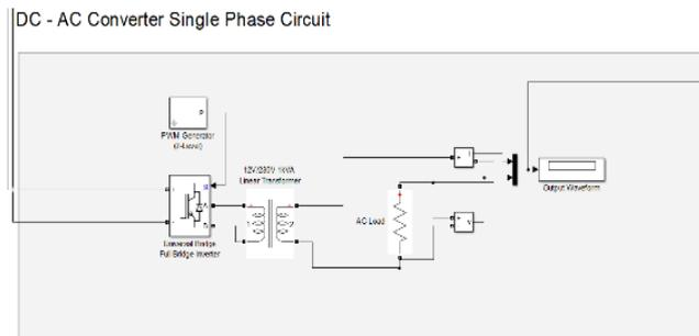
Figure 4. Block Diagram of DC-AC Converter
